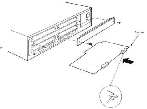
For removal, pull out in direction of arrow so that the ejectors can stay up.
